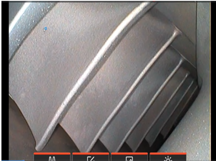
General view of CT blades and Shroud Segments.
