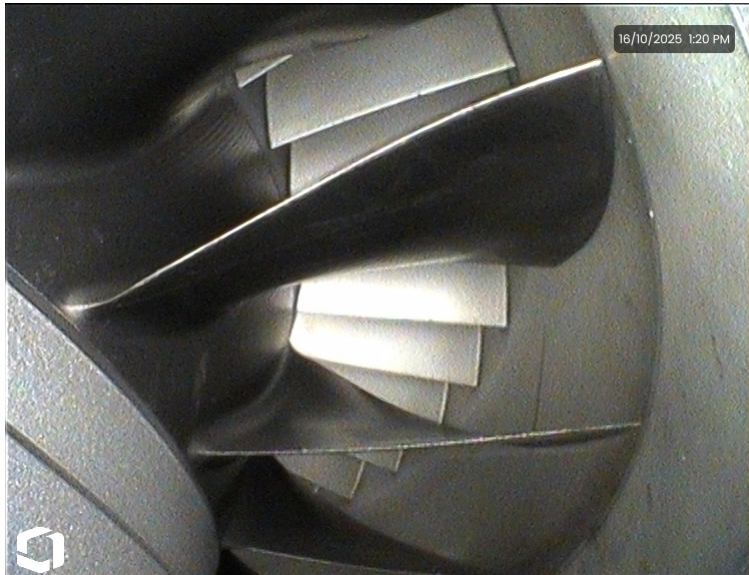
General view on leading edge of First Stage Compressor.
